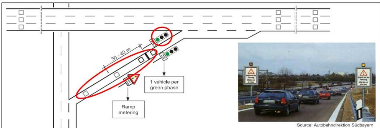
**Figure 7:** Ramp Metering, Interchange Control System, Munich [6]
