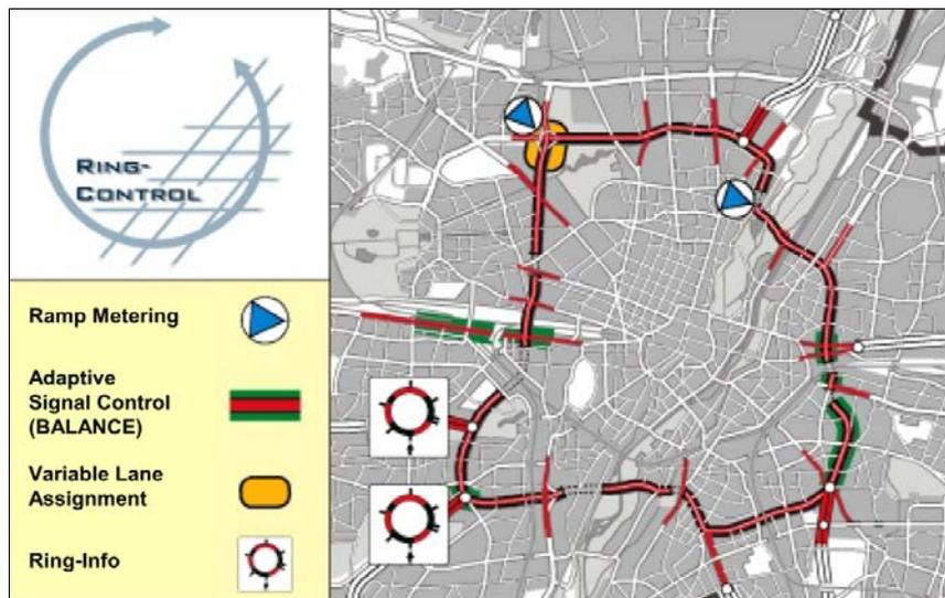
**Figure 8:** ITS Measures for Ring Road Control, Munich [2]
