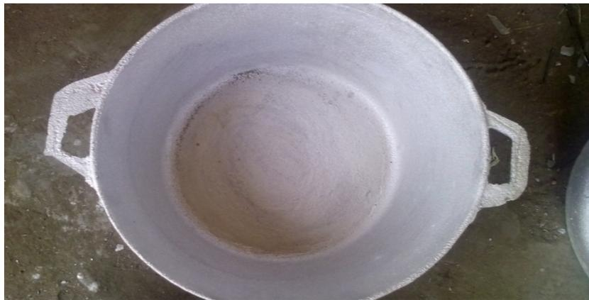
**Figure 3:** Cast Aluminum Plate from Moulding Sand with less than 3% Moisture Content
