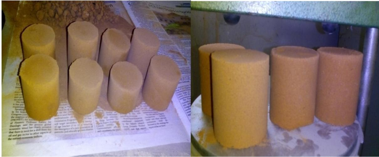
**Figure 1:** Sample Prepared for Moisture Content < 3% **Figure 2:** Sample prepared for test at Moisture content above 3%
