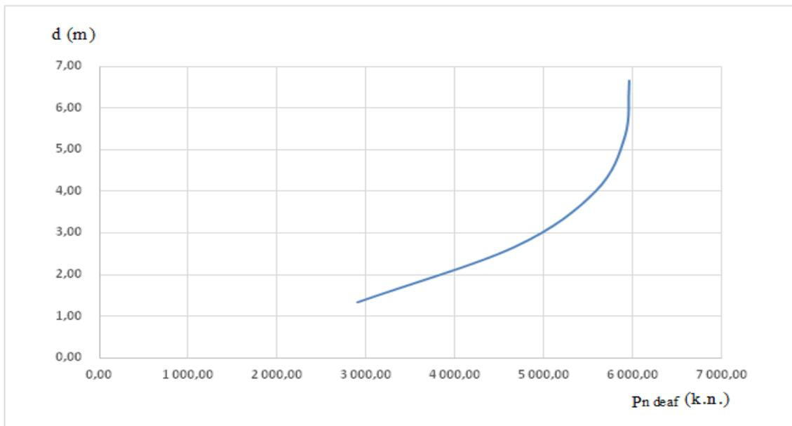
**Figure 6:** The functional dependence between changeable diameter of cylinder shape elements and residual attacking force of debris flow action on the deaf section of the construction after pass through type debris flow against construction
