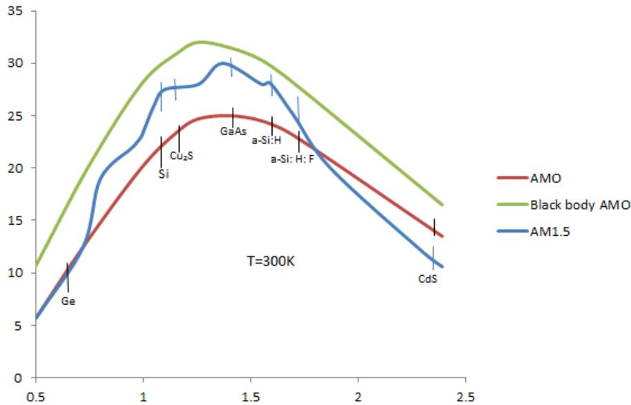
**Figure 6:** Relation between conversion efficiency and semiconductor band gap
