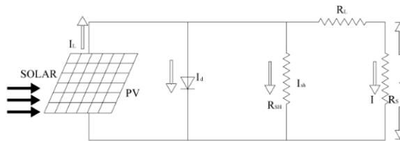
**Figure 2:** Equivalent circuit of PV cell
