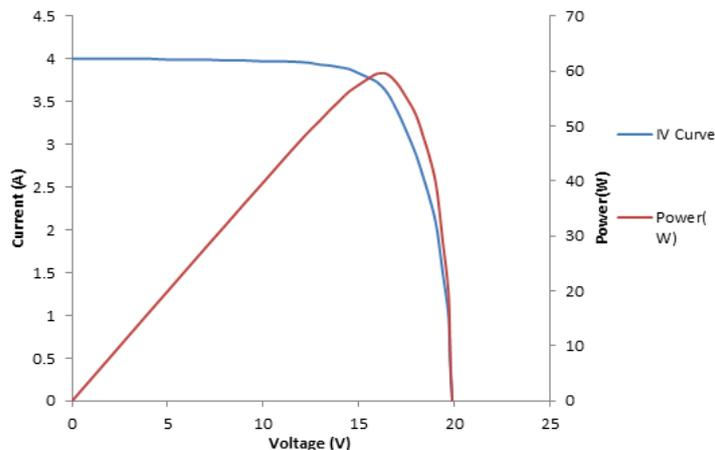
**Figure 3:** IV and PV curves of a silicon module
