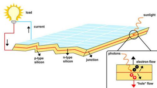
**Figure 1:** Schematic typical Solar cell
