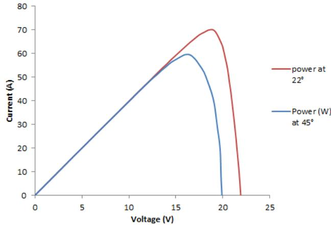
Figure 5: PV curve of solar cell at different temperatures
