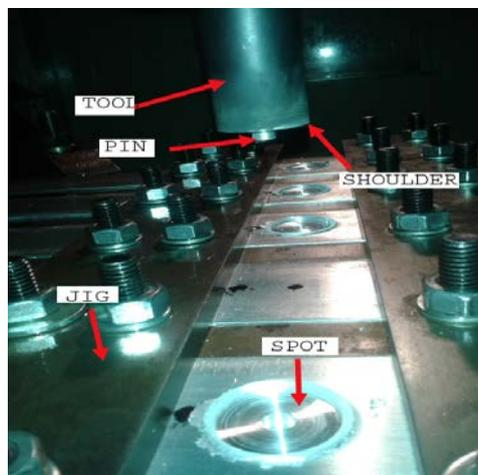
**Figure 1:** The FSSW setup used in the present work.
