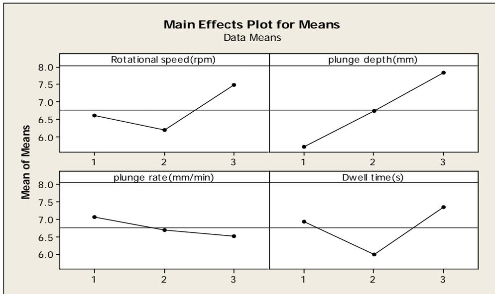
**Figure 3:** Main effects of means of tensile-shear load.
