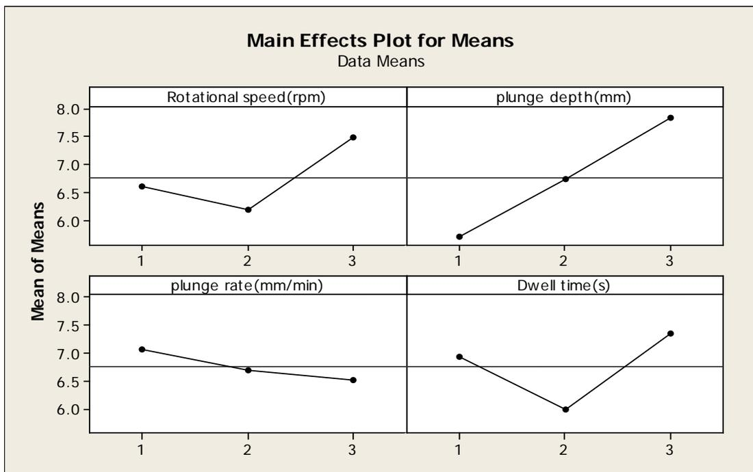
**Figure 2:** Main effects of S/N ratios of tensile-shear load.
