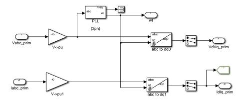
Figure 12: Phase Locked Loop synchronization unit
