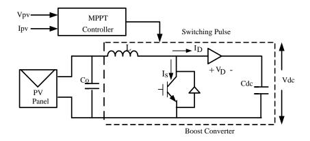
Figure 5: Circuit diagram of DC-DC boost converter [9]
