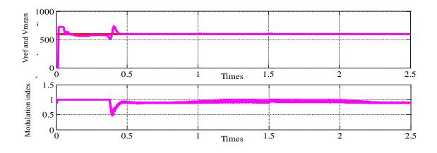
Figure 19: DC link capacitor voltage and modulation index
