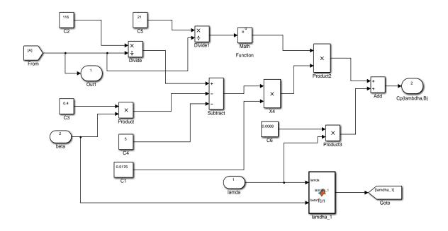
**Figure 4:** Simulink block of performance coefficient Cp  $(\lambda,\beta)$
