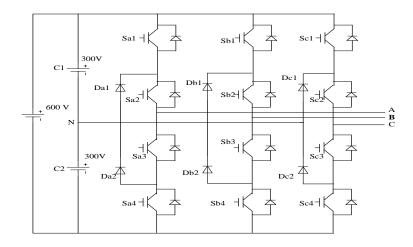
Figure 8: Three phase three level voltage source inverter
