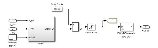
Figure 7: MPPT simulink model
