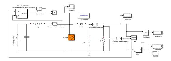
Figure 6: Simulink model of DC-DC boost converter
