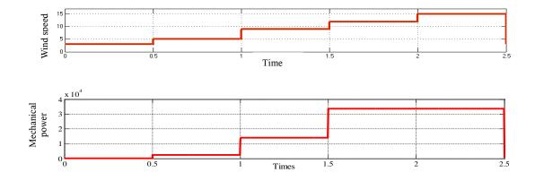
Figure 17: Simulation results for mechanical power output according to different wind speeds
