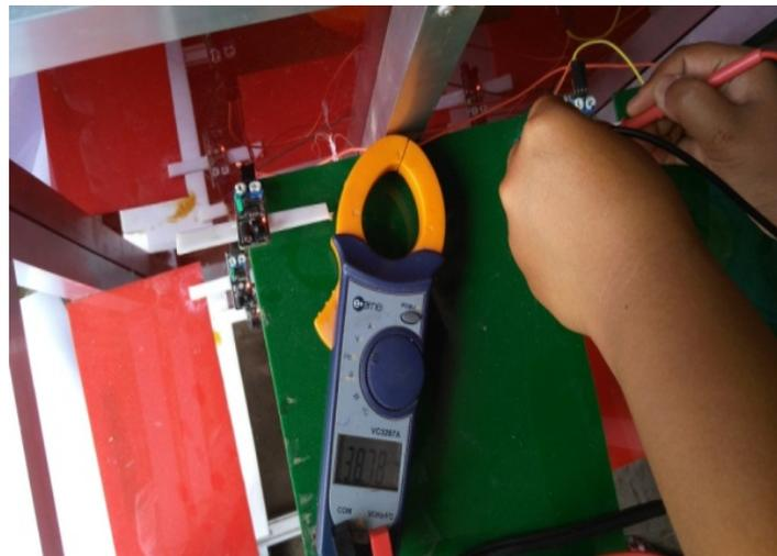
**Figure 12:** Signal Received by IR Obstacle Sensor with frequency 38.78kHz
