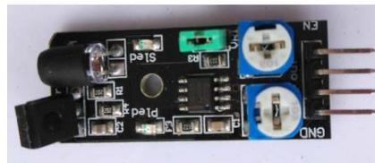
**Figure 4:** Infra-red (IR) Obstacle Avoidance Sensor Module
