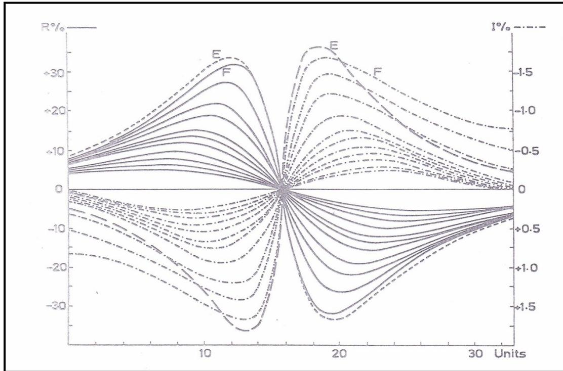
**Figure 17:** VLF. EM Model Profiles for a Vertical Conducting Brass Sheet with Depth of Cover Ranging from 0 to 10 Units, (Baker & Myers 1979)
