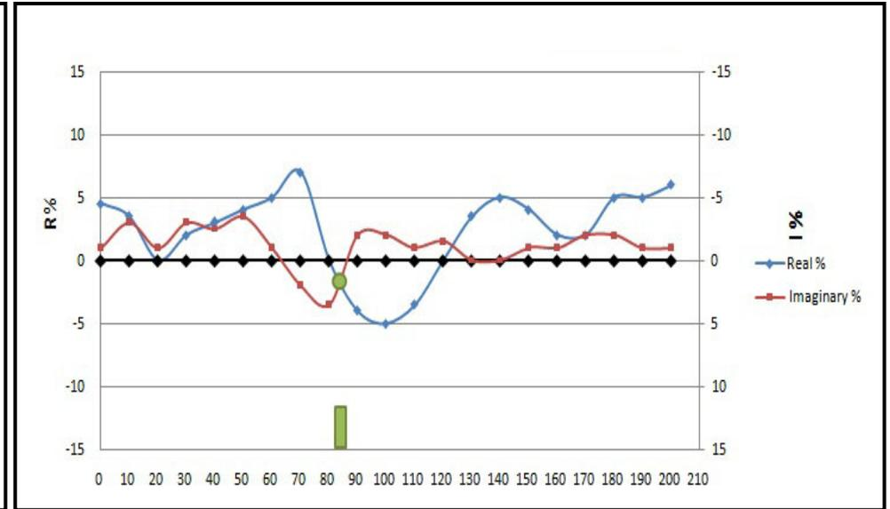
Figure 9: vlf.em profile. Traverse no.5, east, ton=90
