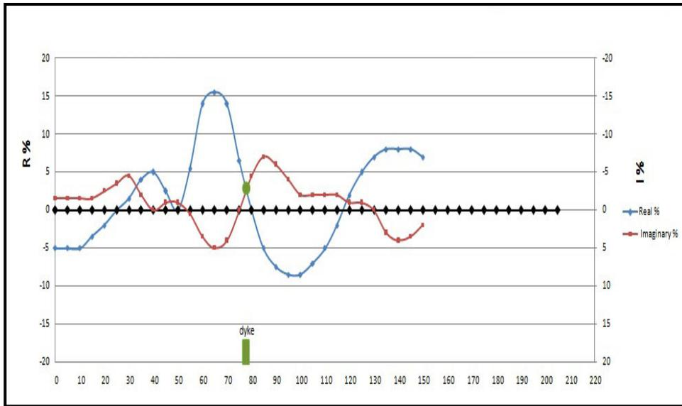
Figure 4: vlf.em profile. Traverse no.1, west, ton=90
