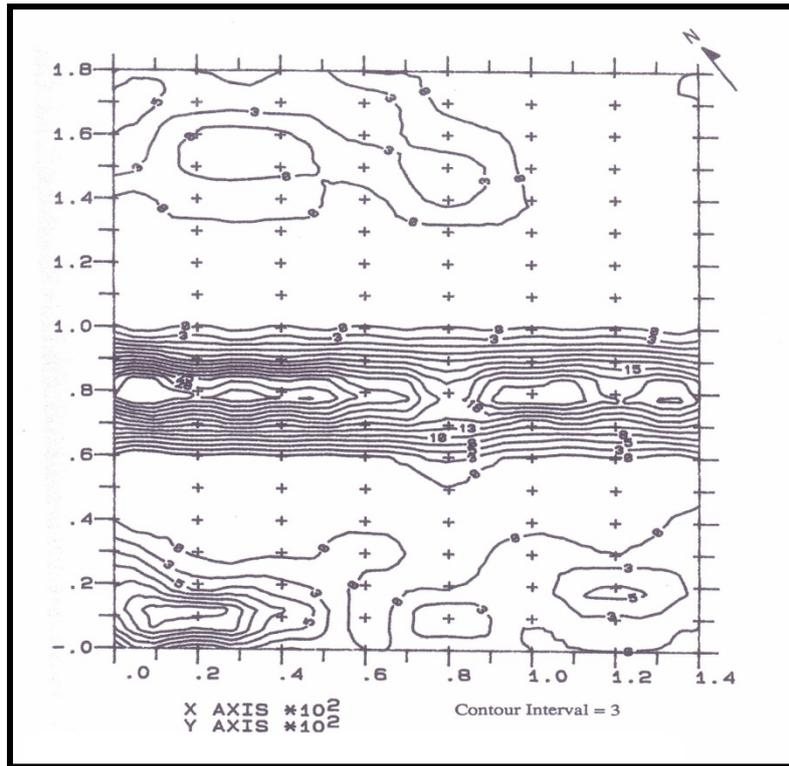
Figure 15: filtered VLF.EM contour map of the studied area
