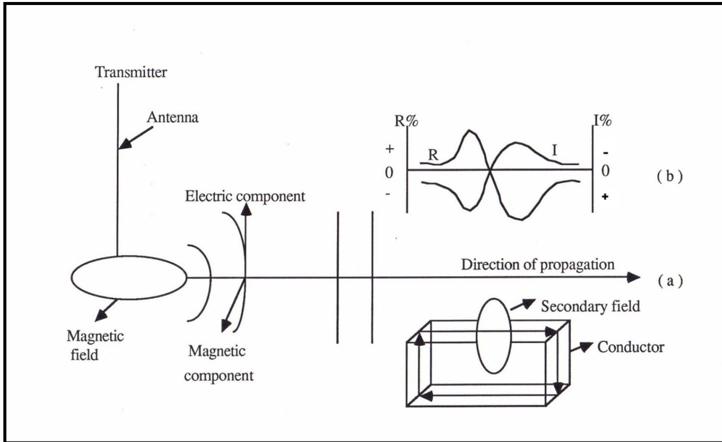
**Figure 2a:** Component and wave propagation associated with the VLF transmitter
