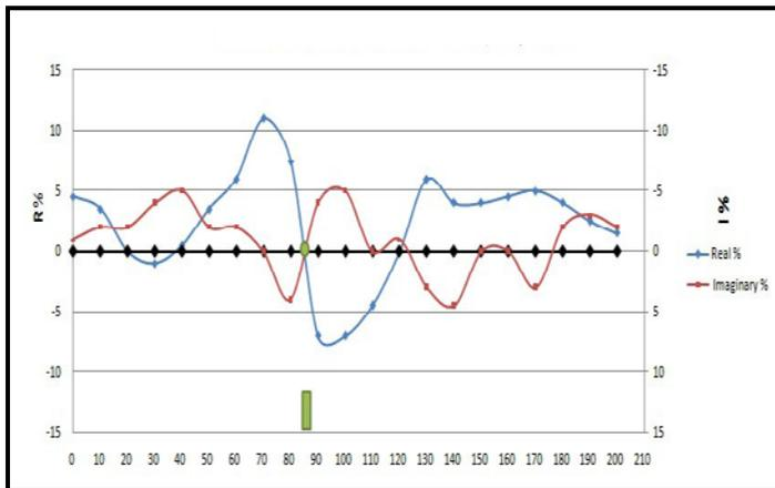
Figure 6: vlf.em profile. Traverse no.2, east, ton=90
