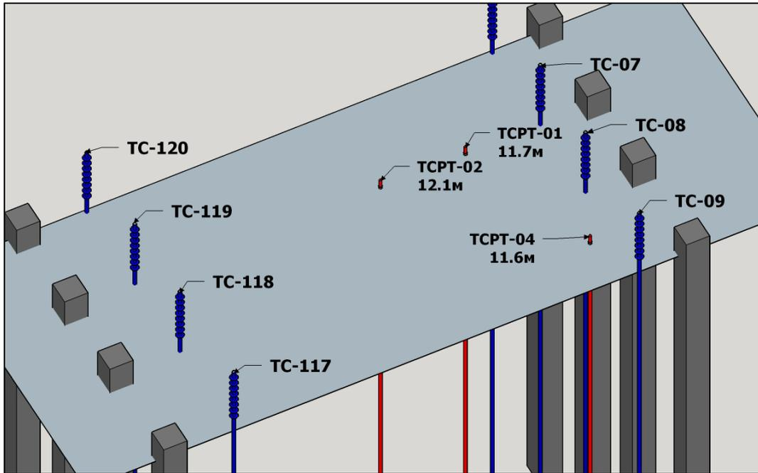
**Figure 6:** Location of Temperature Cone Penetration Tests (TCPT), Thermosyphons (TC) and Piles
