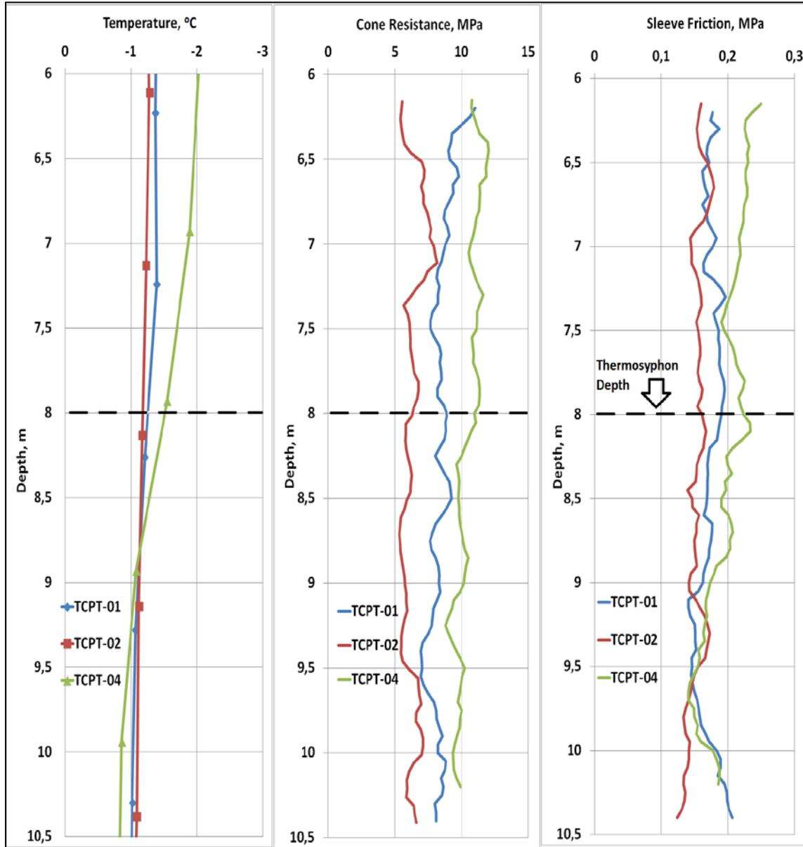
Figure 15: Temperature, Cone Resistance  $q_c$  and Sleeve Friction  $f_s$  vs Depth for EGE-04
