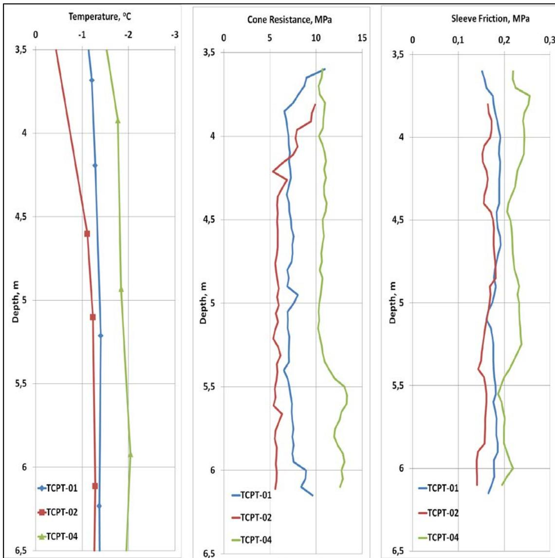
Figure 14: Temperature, Cone Resistance  $q_c$  and Sleeve Friction  $f_s$  vs Depth for EGE-03
