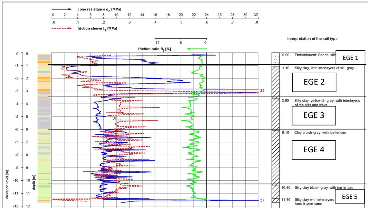
**Figure 8:** EGE discriminated based on CPT and engineering-geological drilling for TCTP-01
