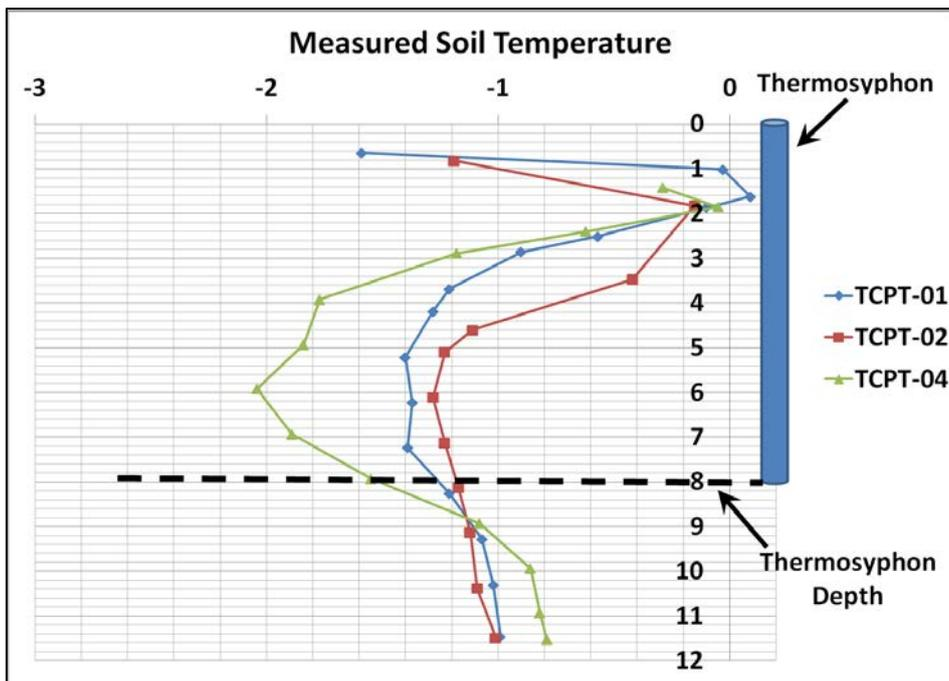
Figure 12: Measured Soil Temperature Profiles at TCPT-01, TCPT-02 and TCPT-04
