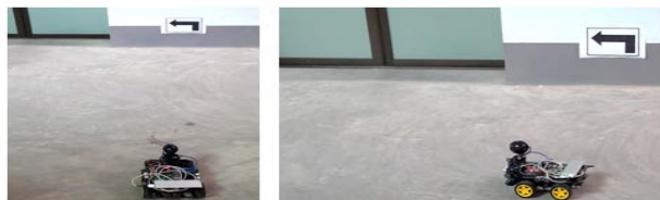
Figure 19: Detect Turn Right Sign landmark and turn
