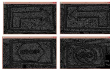
Figure 8: Processing results for Canny edge detection
