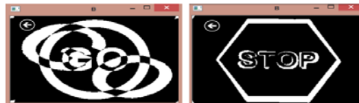
Figure 11: Processing results for matching landmark using XOR
