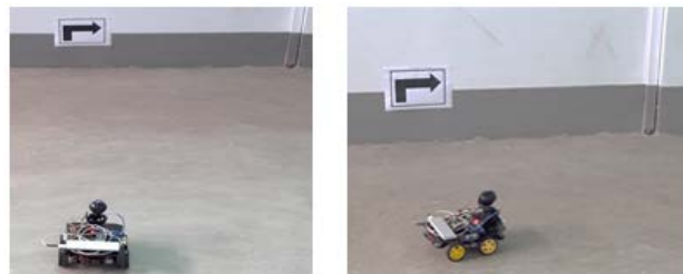
Figure 18: Detect Turn Right Sign landmark and turn
