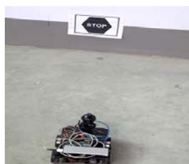
Figure 20: Detect Stop Sign landmark and then stop
