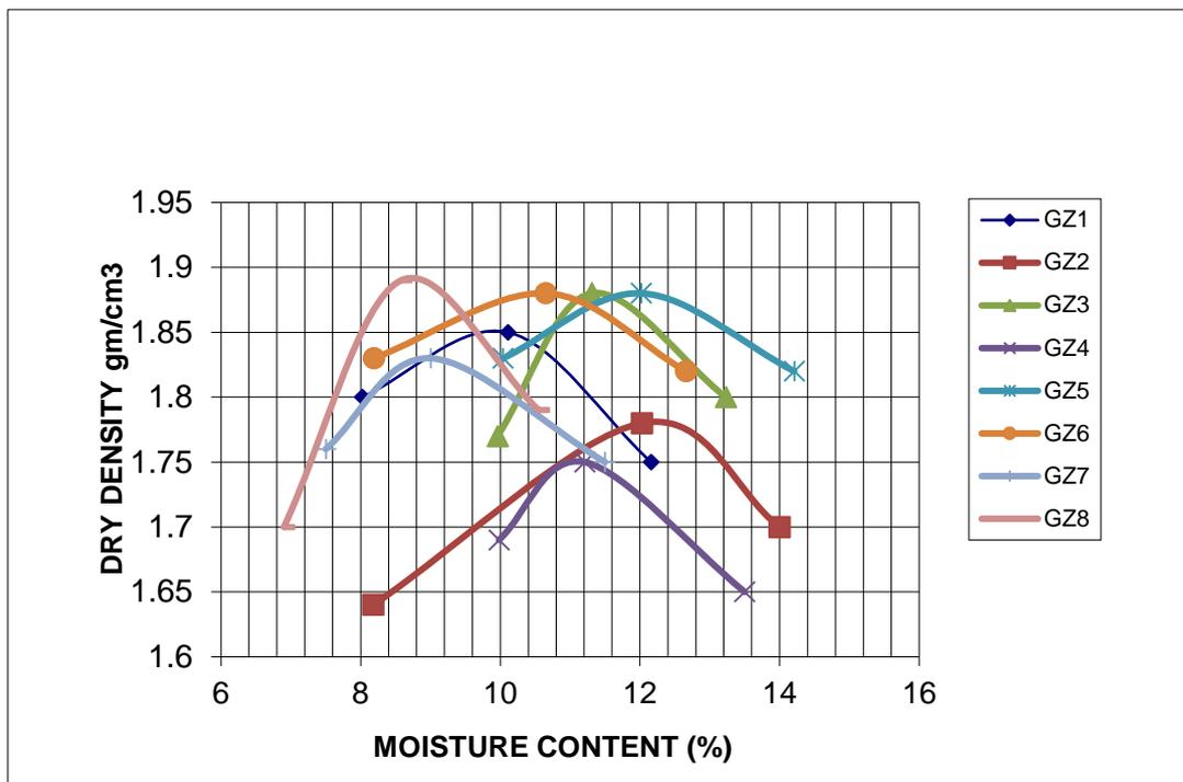
**Figure 11:** Compaction curve for all samples
