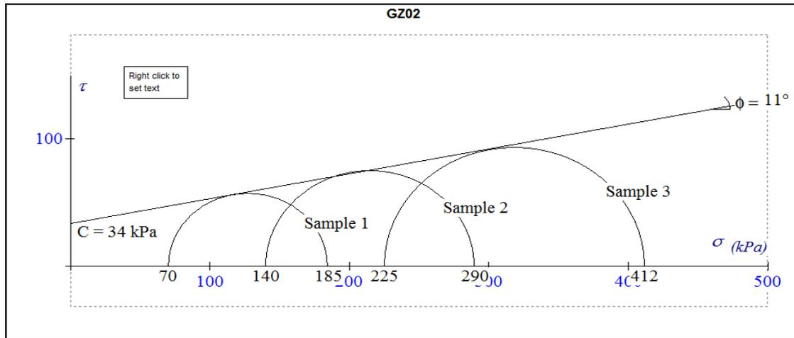
Figure12: a: Morh view plot for crack zone.
