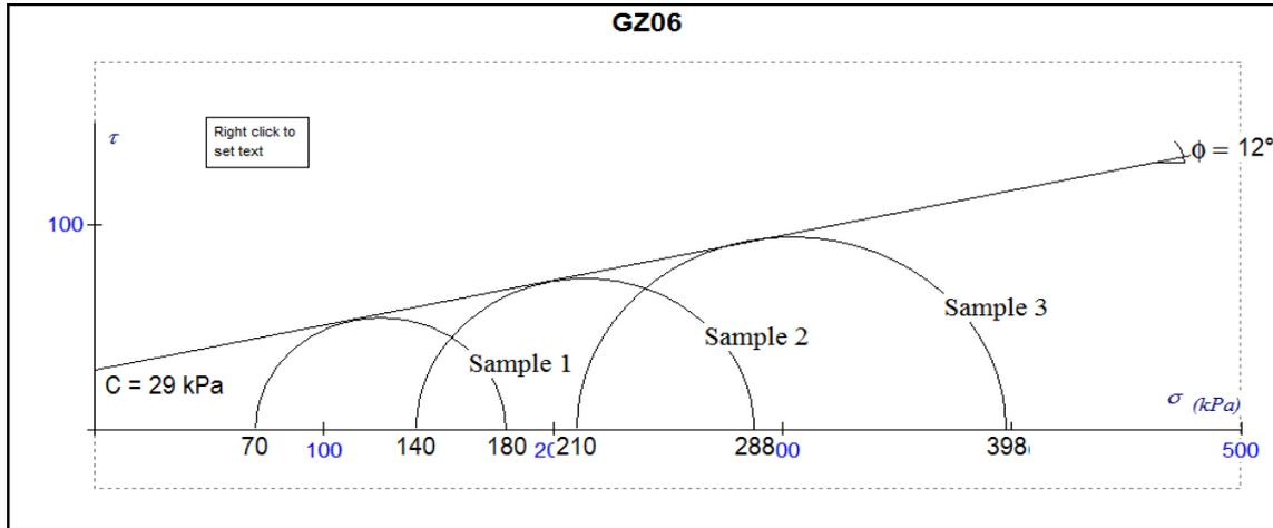
Figure 12b: Morh view plot for non-cracked zone
