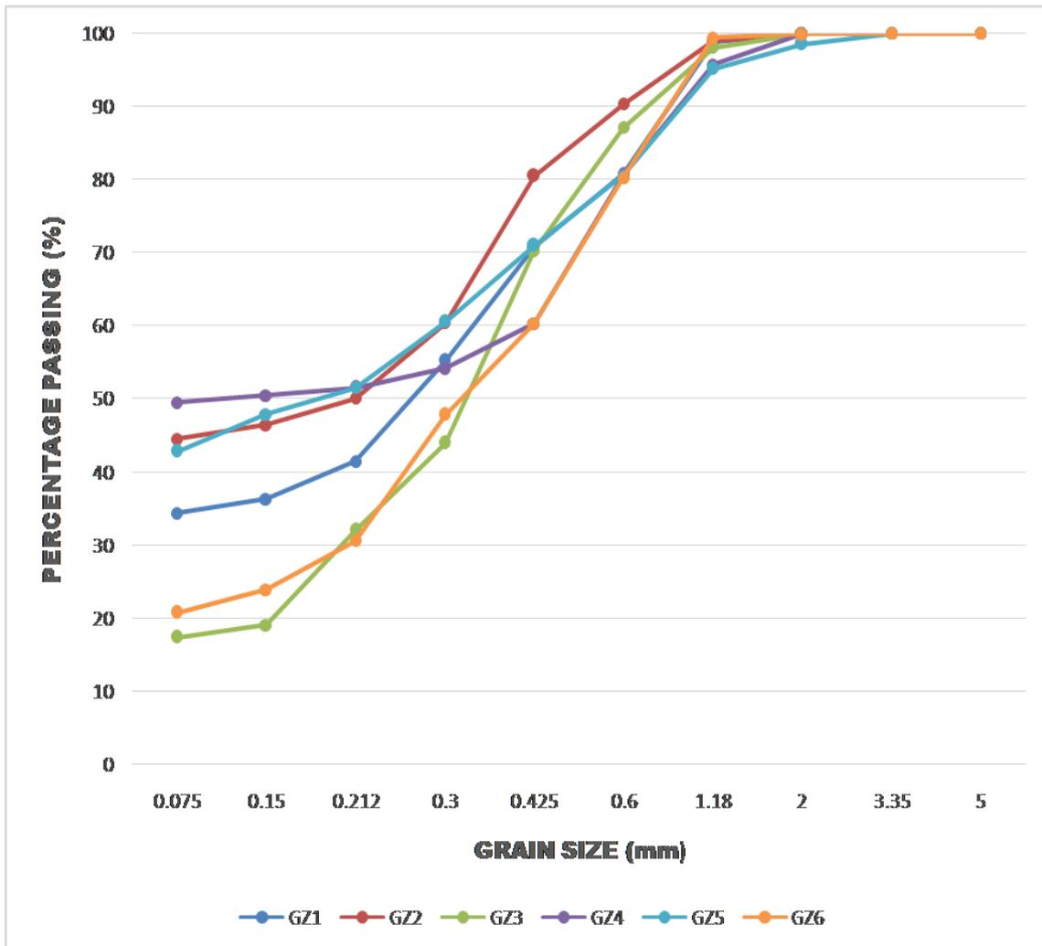
Figure 8: Grain size distribution curve
