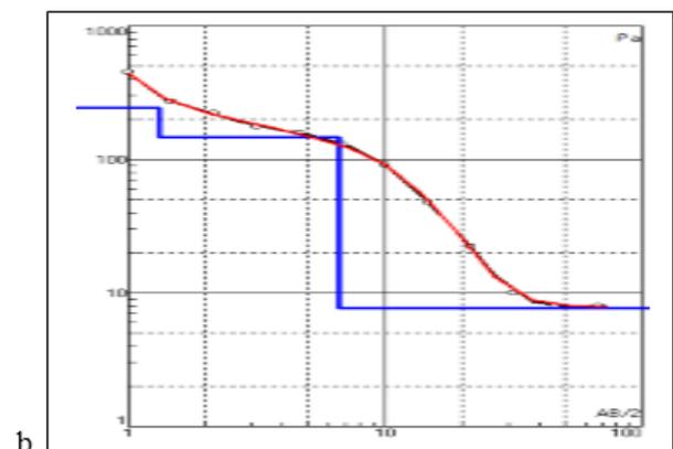
**Figure 7:** 1-D resistivity model curves of the study area: (a) for VES 1, and (b) for VES 4
