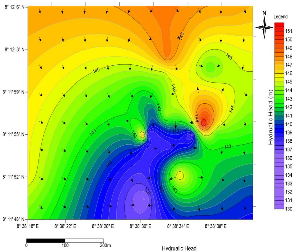
Figure 13: Hydraulic head map showing direction of groundwater flow
