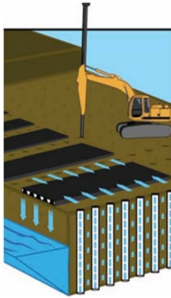
Figure 3: Increased horizontal permeability and the short distance between the piles greatly limit the time of consolidation (Source: Kaltzios 2012, [3] Platis-Vgenopoulou 2016, [7])
