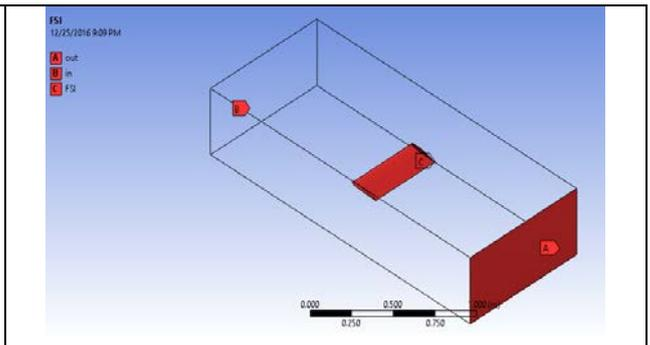
**Figure 3:** Named sections of fluid domain
