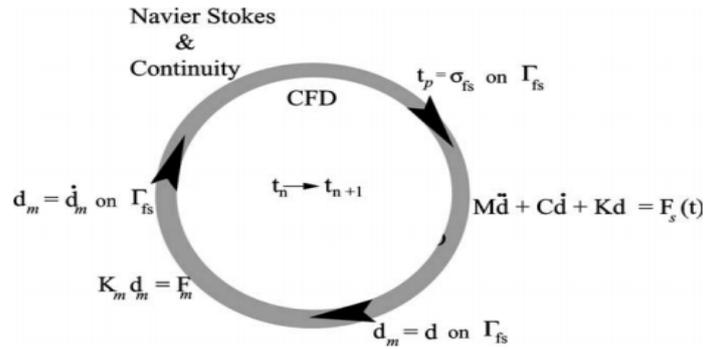
**Figure 1:** dynamic fluid structure interaction analysis systems[21]
