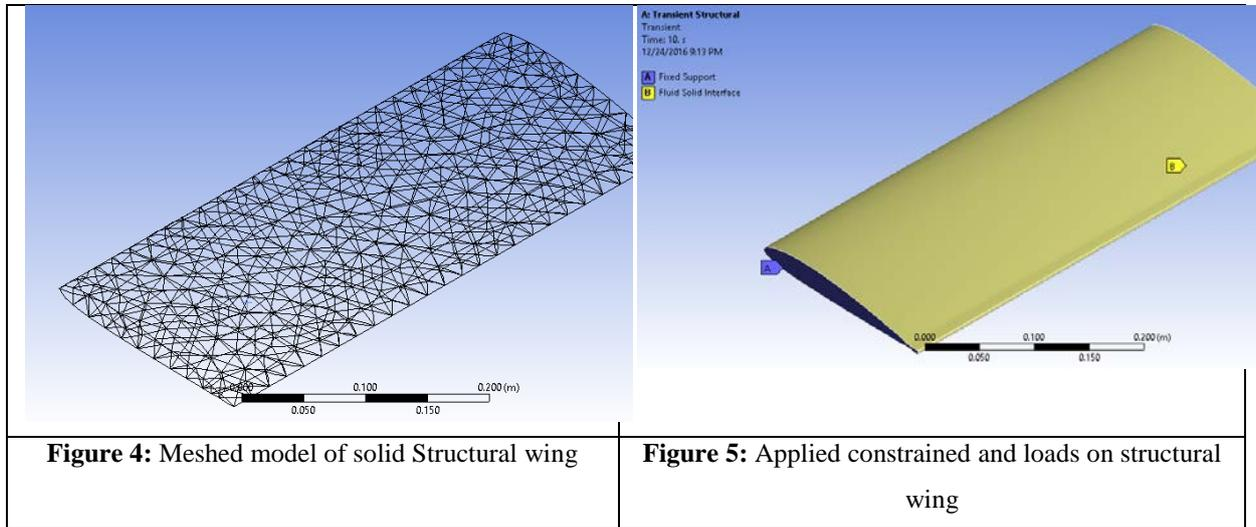
**Figure 4:** Meshed model of solid Structural wing
