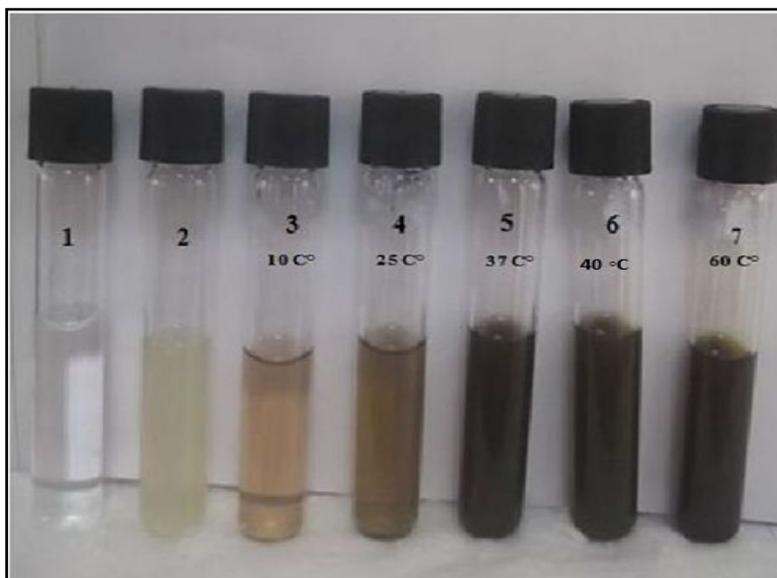
**Figure 6:** Digital photograph shows different colors obtained through the silver reduction assay at different temperatures , indicating silver nanoparticle formation. The tubes(3-7) represent
