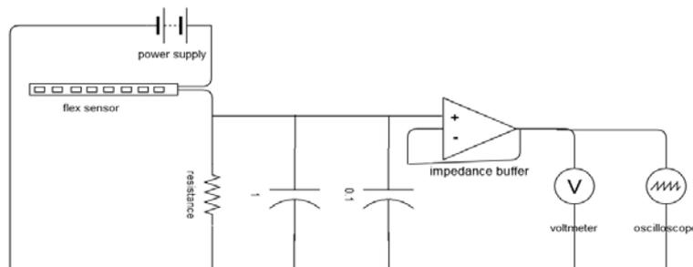
**Figure 12:** the second electrical circuit for flex sensor
