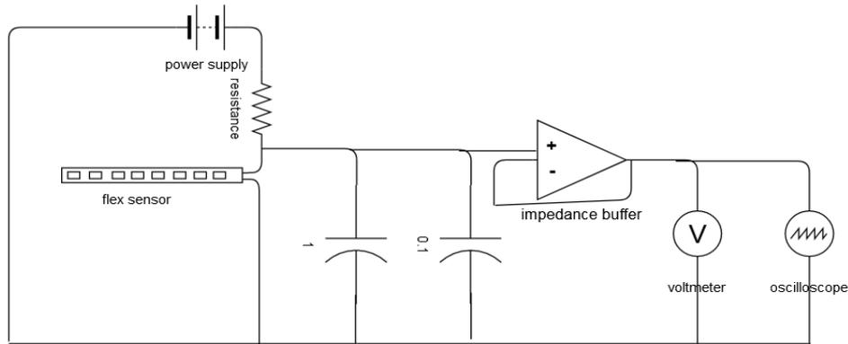
**Figure 11:** the first electrical circuit for flex sensor
