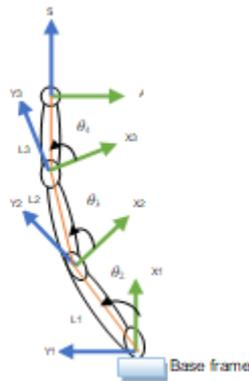
**Figure 7:** projection of the finger onto  $x_0-y_0$  Plane.
