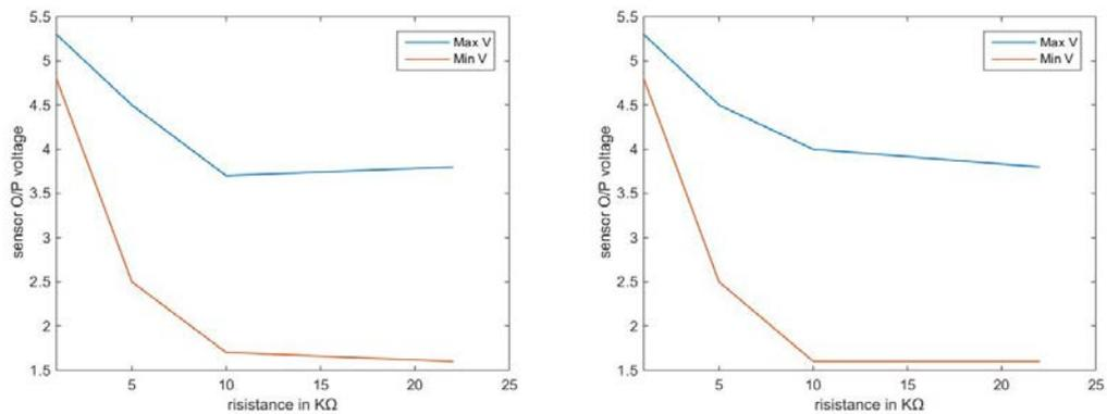
**Figure 13:** range of the output voltage for circuit 1 and 2.
