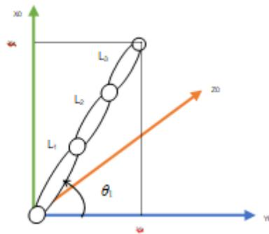
**Figure 6:** projection of the finger onto  $x_0-z_0$  plane.
