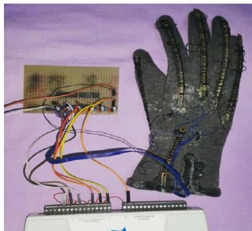
**Figure 9:** sensory glove hardware circuit
