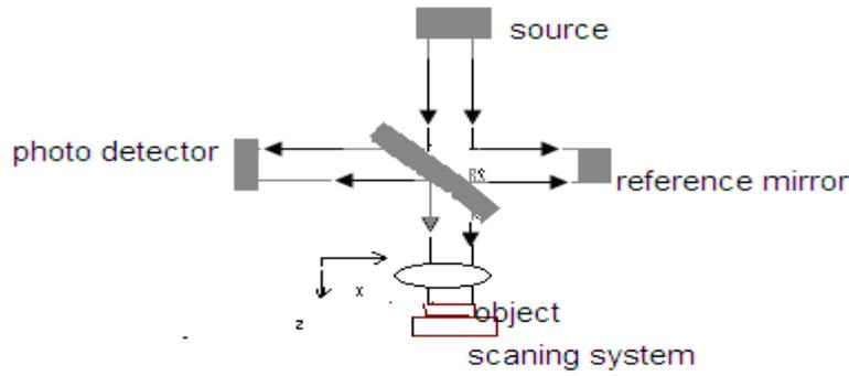
**Figure 1:** block diagram of the constructed (OCT) system
