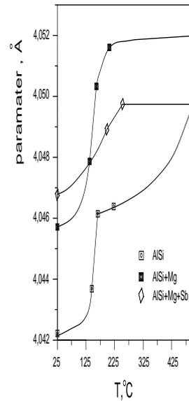
**Figure 1:** Change of lattice parameter of Al matrix after isothermal annealing
