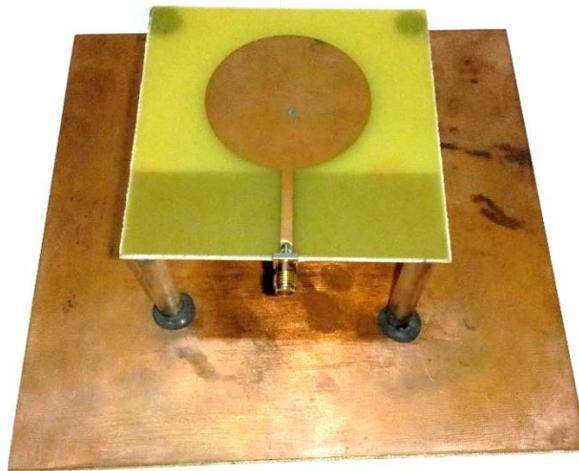
**Figure 9:** The fabricated UWB antenna.
