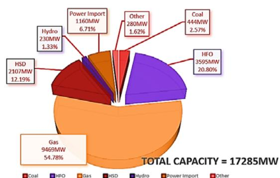
**Figure 11:** Fuel wise de-rated power generation capacity (MW) of Bangladesh (installed capacity of BPDB power plants as on October 2018) in year 2018 [11]
