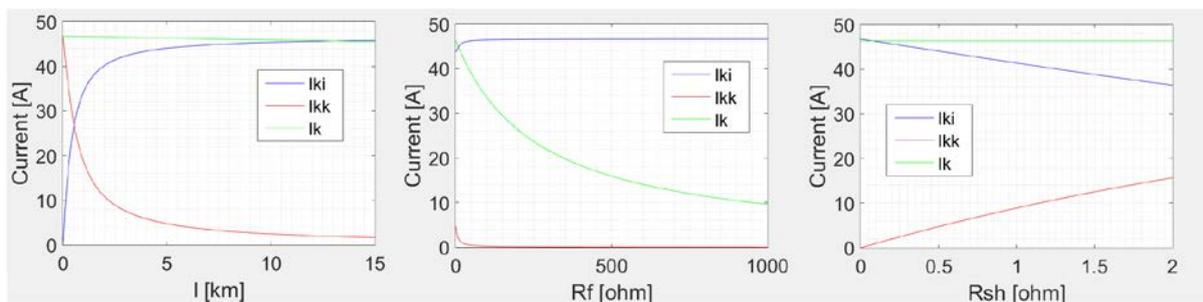
Figure 9: Dependences of the fault currents model without load - compensated earthing
