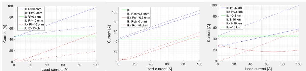
Figure 10: Dependences of the fault currents on line load - compensated earthing
