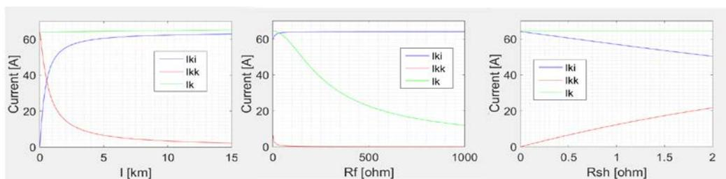
**Figure 5:** Dependences of the fault currents model without load - isolated network
