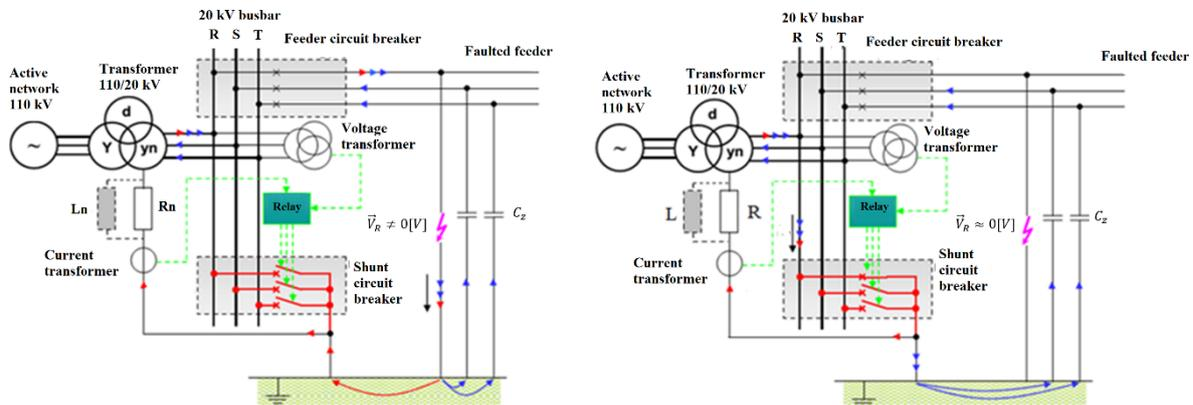
**Figure 1:** Operation principle of shunt circuit breaker left (off), right (on)
