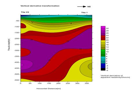
Figure 7: Pseudo-section of vertical derivative transformation
