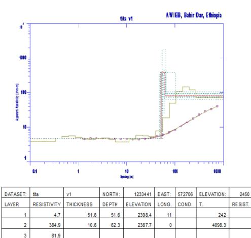
Figure 14: Data inversion model of TITA V1
