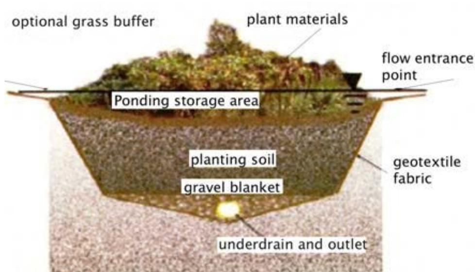
**Figure 3:** Typical Illustration for Bioretention Area
