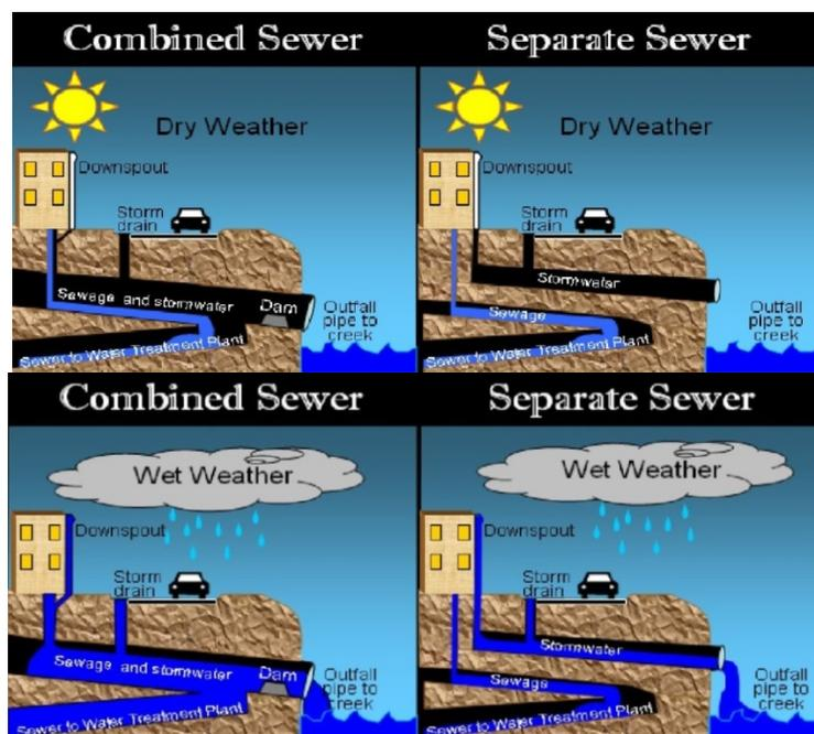
**Figure 2:** Typical Illustration of Combined Sewer Overflow and Separated System
