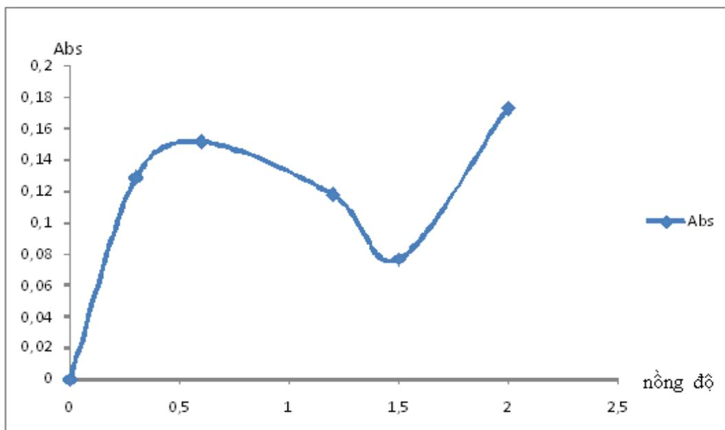
**Figure 7:** The effects of  $KMnO_4$  concentration on reaction
