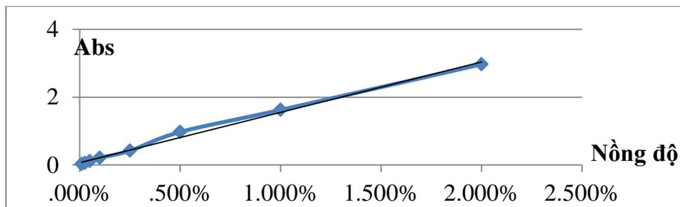
Figure 5: The relationship between methanol concentration in gasoline and optical absorption at concentrations between methanol 0.5% and 2.5%.
