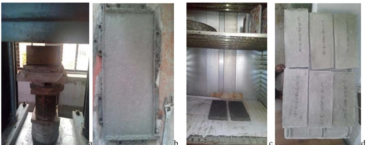
**Figure 2:** Applying pressure (a) on cement board; (b) after removal; (c) Curing in Oven and (d) at room environment
