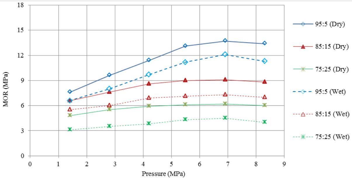
Figure 3: Relation between Paper content, Pressure and Modulus of Rupture (MOR)
