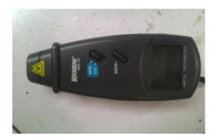
Figure 6: Tachometer
