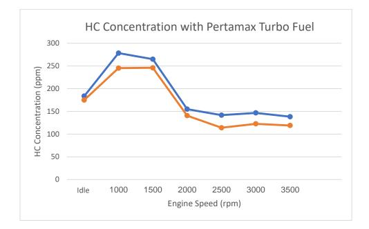
Figure 12: HC concentration in pertamax turbo fuel with variations in engine speed
