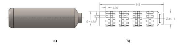
Figure 4: (a) casing of catalytic converter (b) dimension of catalytic converter core
