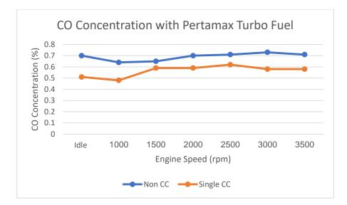
Figure 9: CO concentration in the pertamax turbo fuel with variations in engine speed
