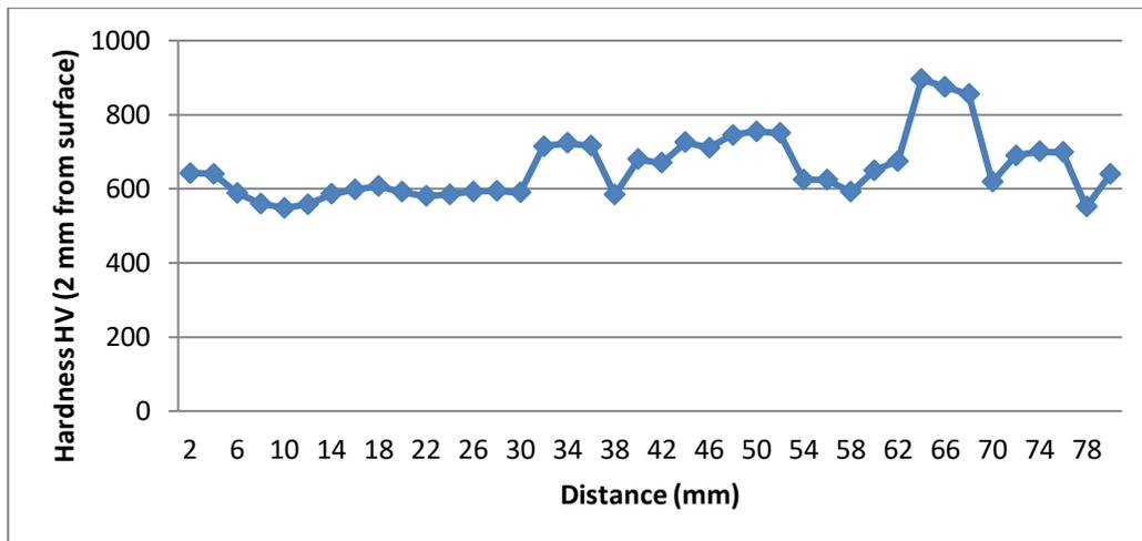
**Figure 9:** Rear Axle Hardness Distribution B
