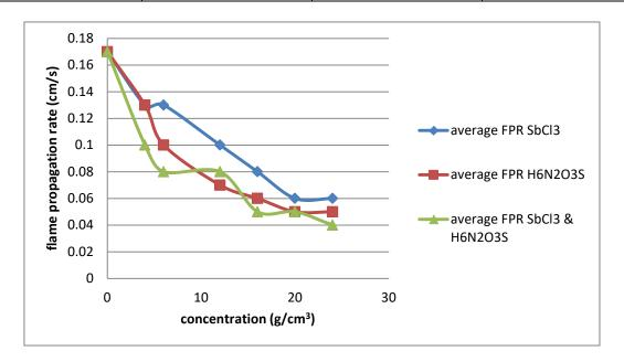
Figure 3: Effect of flame retardants on flame propagation rate of wood splints.
