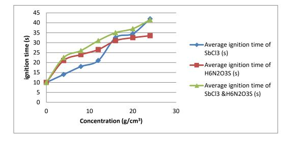
Figure 2: Effect of flame retardants on ignition time of wood splints.
