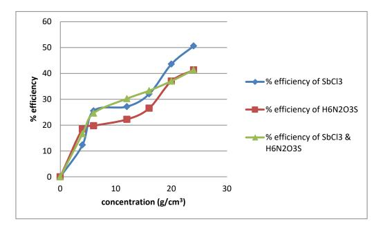
Figure 1: Percentage efficiency of the flame retardants on wood splints
