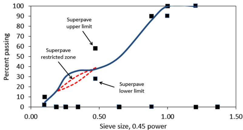
**Figure 4:** Aggregate gradation.
