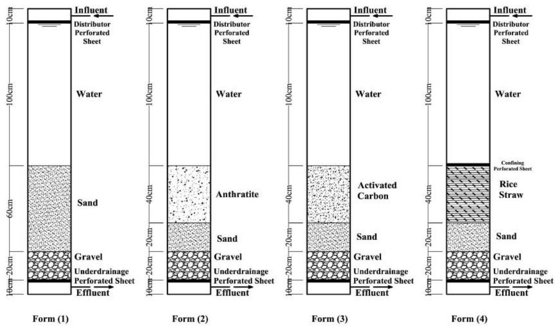
Figure 3: The different arrangements of filter media
