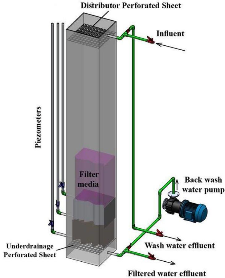
**Figure 2:** The experimental model of the filter
