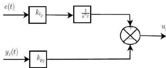
**Figure 13:** Structure of the fractional PI controller
