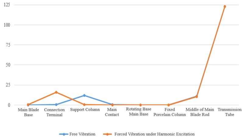
**Figure 4:** Lorenzetti 242 kV high voltage switch deformation.
