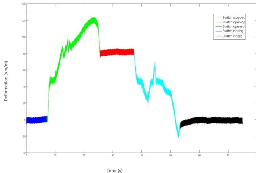
**Figure 5:** Deformation of the Lorenzetti's 242 kV transmission tube.
