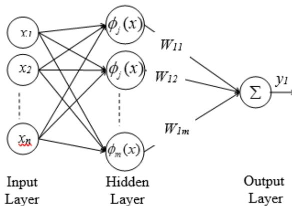
**Figure 2:** Schematic diagram of a RBF network.
