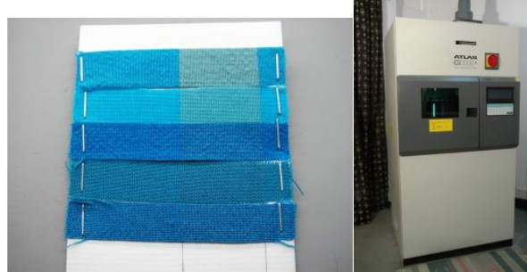
Figure 13: Blue Wool Standards-ISO 105 BO2 Water cooled light fastness testing machine Results of light fastness of traditional printing
