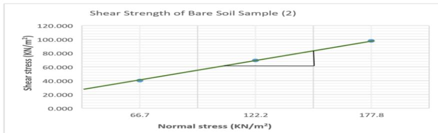
**Figure 5:** Shear strength graph of bare soil sample (2)
