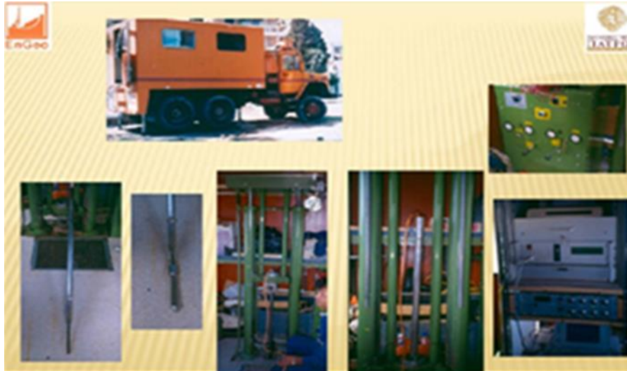
Figure 2: Hydraulic cone penetrometer system [9].
