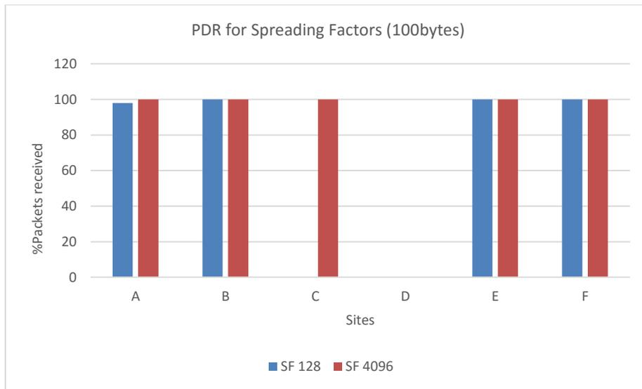
**Figure 8:** PDR for SF=128 and SF=4096 with payload size of 100bytes
