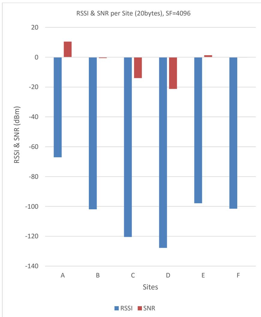
**Figure 9:** RSSI values for payload size of 20bytes
