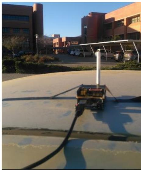
**Figure 3:** Client node mounted on car
