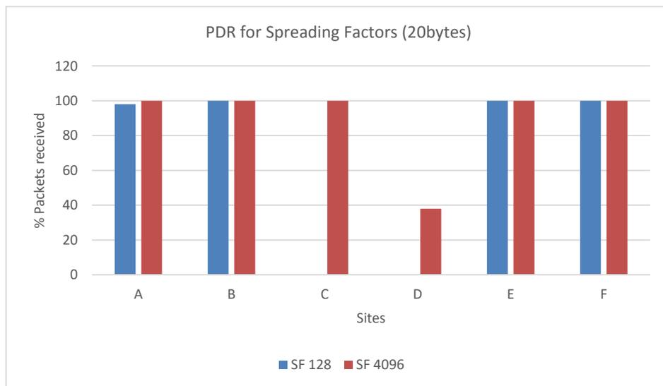
**Figure 7:** PDR for SF=128 and SF=4096 with payload size of 20bytes
