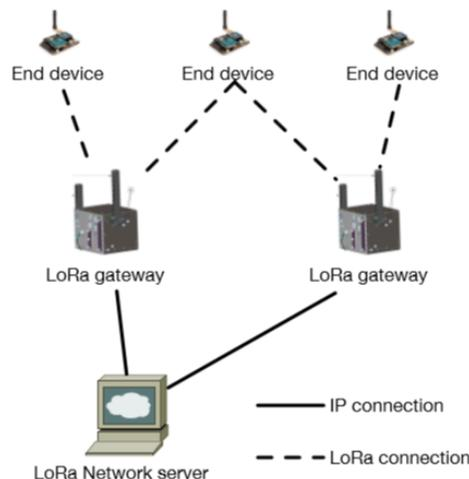
**Figure 2:** LoRaWAN Network Architecture
