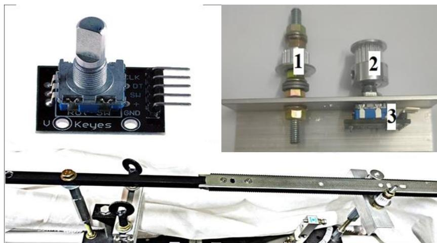
**Figure 3:** (Upper right) the aluminum pulley that used to couple the encoders in a close direction, where (1) refers to the pulley roller and (2) refers to the aluminum pulley while (3) represents the encoder. (Upper left) the encoder type that used to convert the linear motion of actuators into a corresponding electrical signal. (Lower) the metallic bar and the belt that used to restrict direction of the movement.
