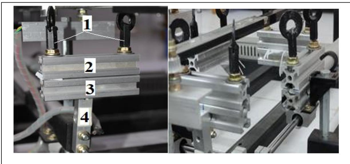
**Figure 2:** Manufactured grippers which consists of a screw (1), upper part (2), lower part (3), and the load cell (4).
