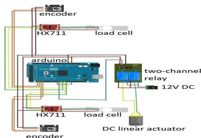
**Figure 4:** The electric circuit of the shield of HX711 that was used in the fabricated 2DTTD enables the Arduino mega controller to sense load cell signals.
