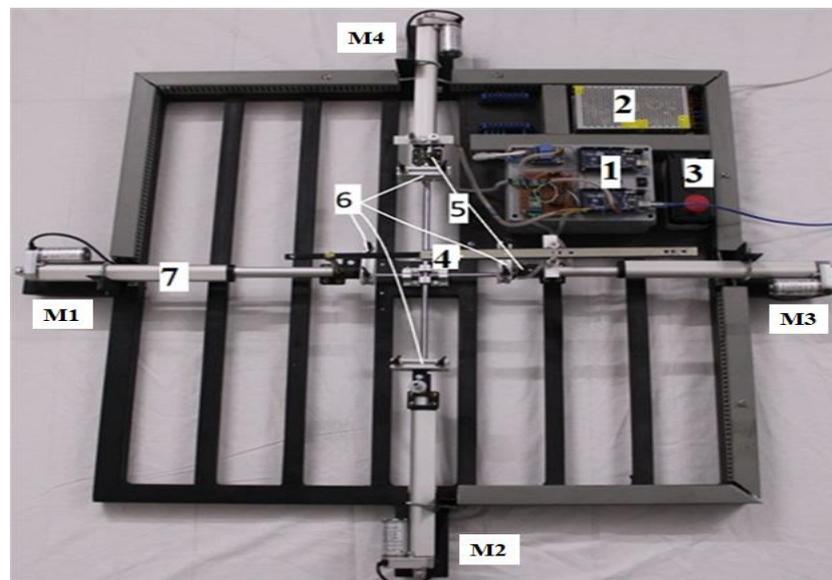
**Figure 1:** The main elements of the experimental set-up. Four independent linear DC motors [hydj12-250]. 1 represents the control circuit. 2 represents the control power supply. 3 represents the emergency switch. 4 represents the encoder guid. 5 represents two-load cells. 6 represents Four-grippers. 7 represents the DC linear actuator.
