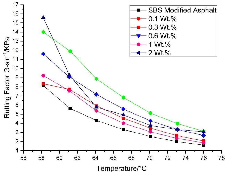
Figure 1: SBS Modified asphalt rutting factor
