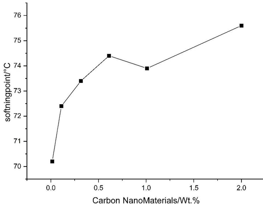
**Figure 2:** SBS Modified Asphalt softening point of carbon nanomaterials
