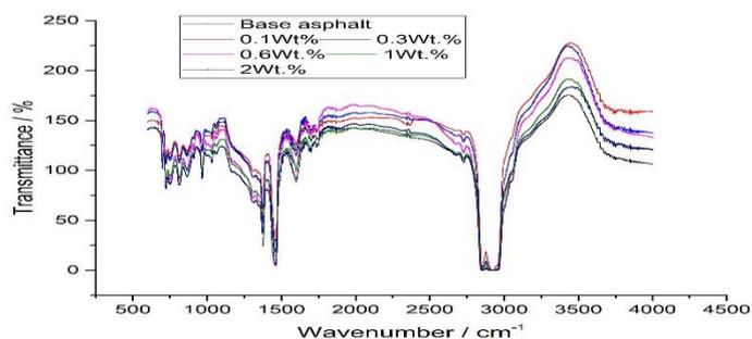
**Figure 7:** infrared spectroscopy of/SBS modified asphalt for carbon nanomaterials
