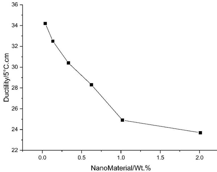
**Figure 3:** Carbon nanometer/SBS modified asphalt extension test
