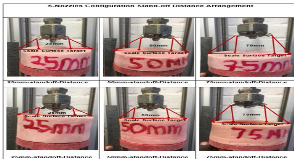
Figure 2. 7: Stand-off distance arrangement [39].
