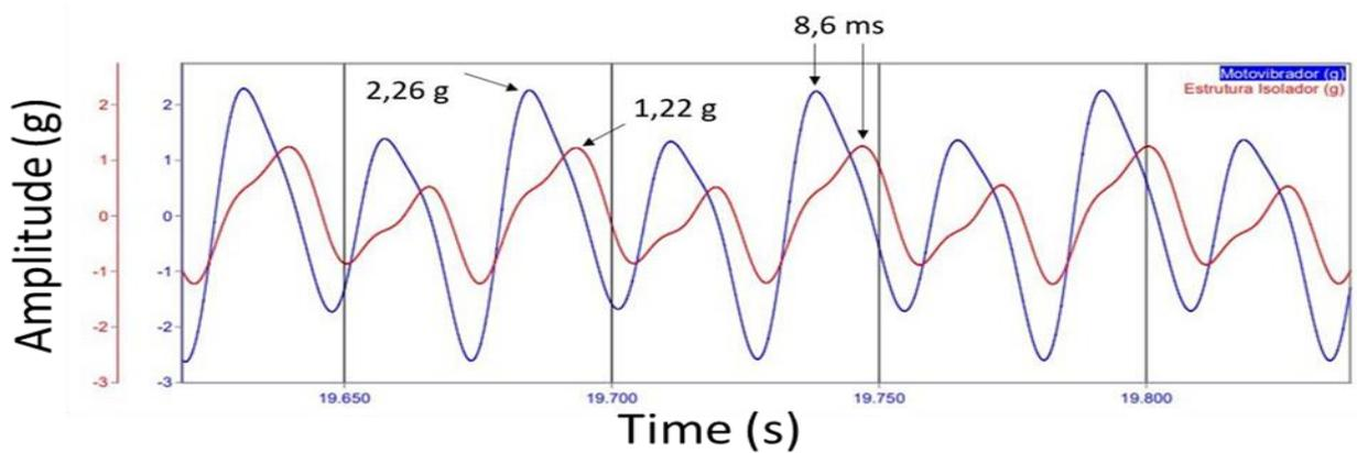
**Figure 15:** Comparison of the vibration from the vibrator (blue) and insulators' base (red)
