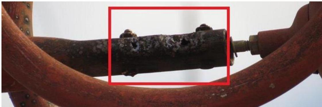
**Figure 2:** Problem in contacts due to bad closing
