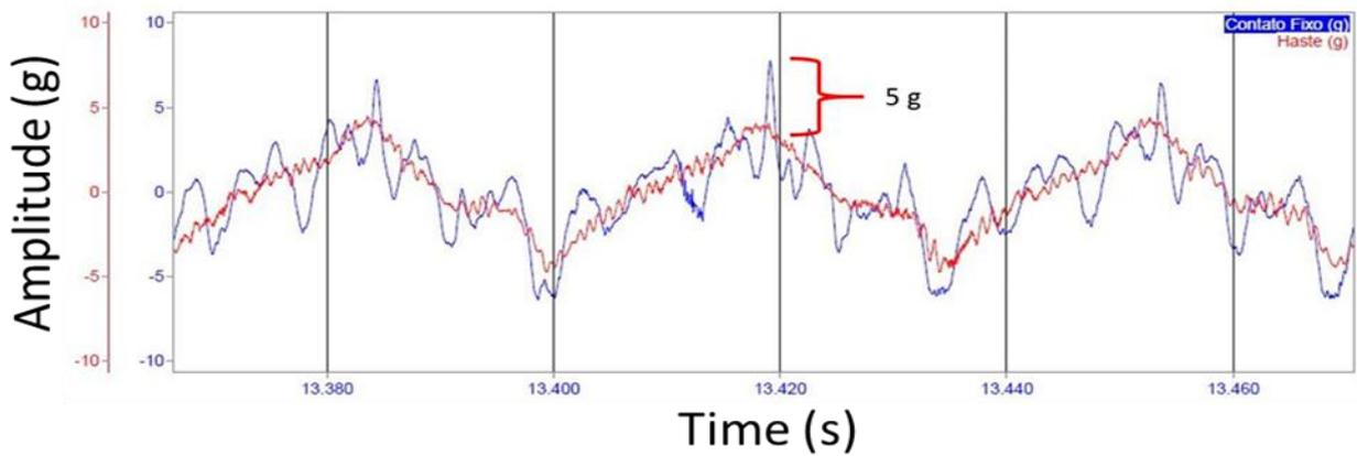
**Figure 14:** Comparison between 34Hz contacts, mobile contact (red) and fixed contact (blue)
