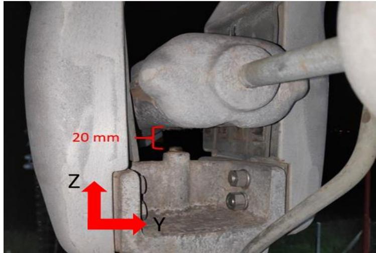
**Figure 6:** Contact opening (20mm opening)
