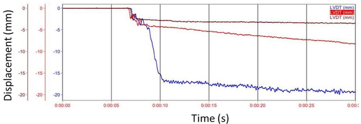
**Figure 18:** LVDT general displacement – 24Hz (brown), 34Hz (red), 43,5 Hz (blue)
