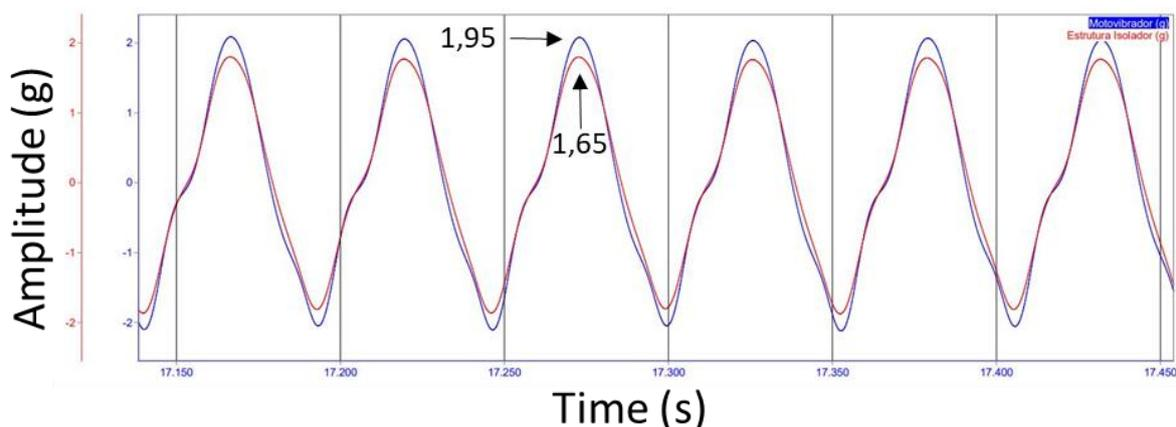
**Figure 9:** Comparison between the vibration of the vibrator (blue) and the base of the insulators (red) in 24Hz
