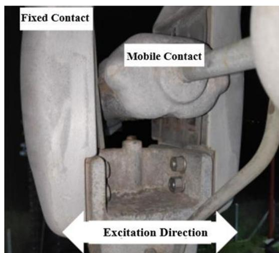
**Figure 3:** Direction of excitation in relation to contacts
