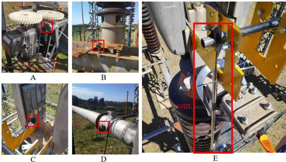
**Figure 7:** Positioning of accelerometers
