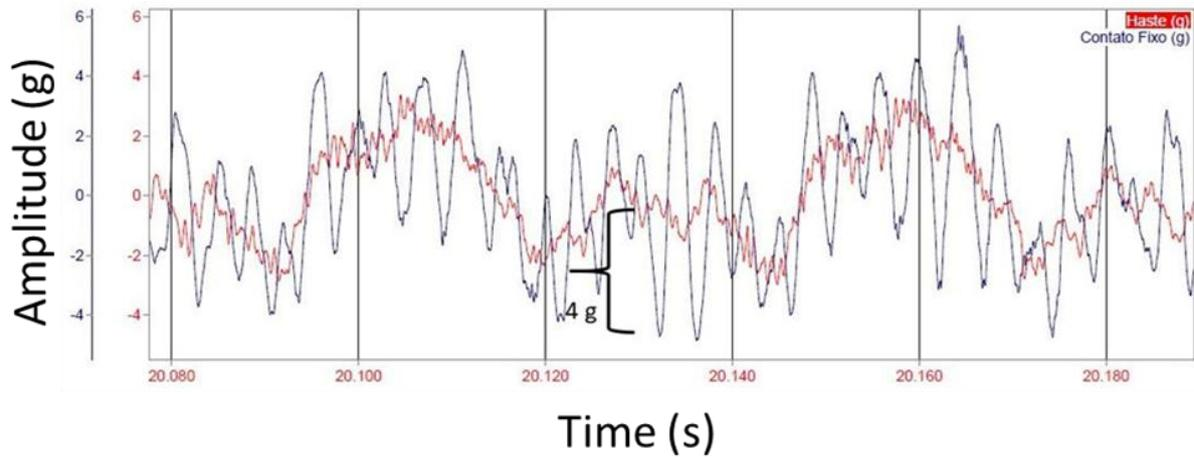
**Figure 11:** Comparison between 24Hz contacts, mobile contact (red) and fixed contact (blue)
