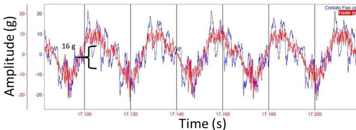
Figure 17: Vibration in fixed contacts (blue) and mobile contacts (red)
