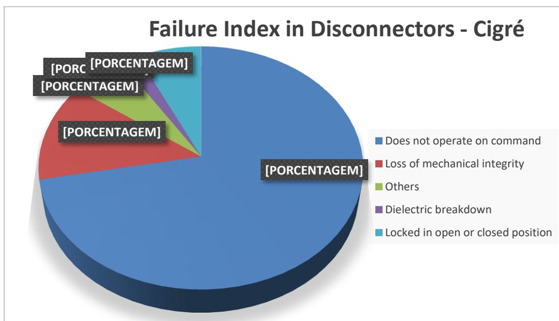
**Figure 1:** Failure index in disconnectors
