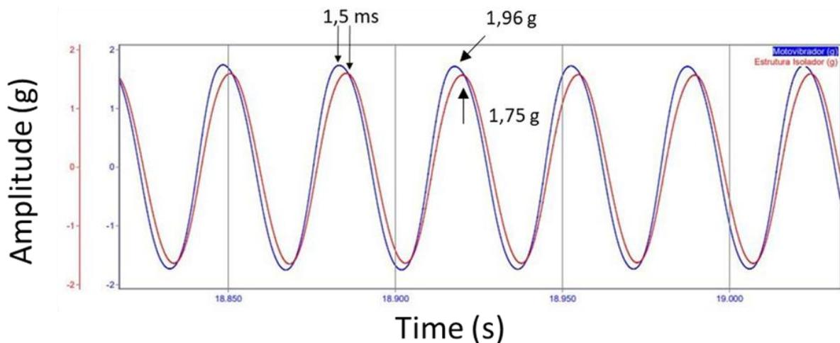
**Figure 12:** Comparison of the vibration from the vibrator (blue) and insulators' base (red) at 34Hz
