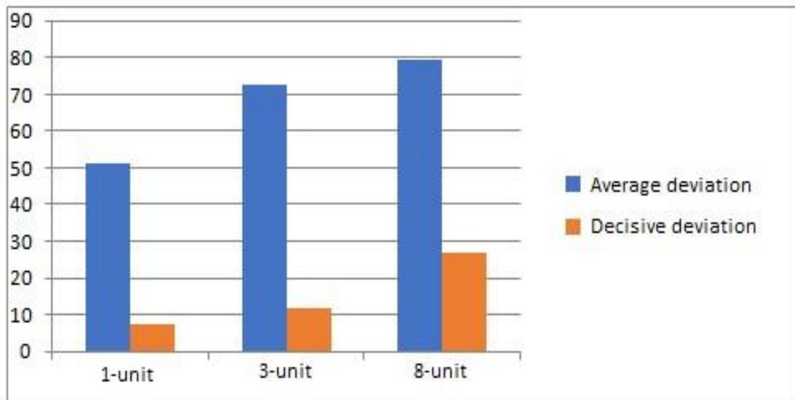
**Figure 4:** Graphic representation of the deviation of 3D and milled samples with aspect to the size of work in [ $\mu\text{m}$ ]
