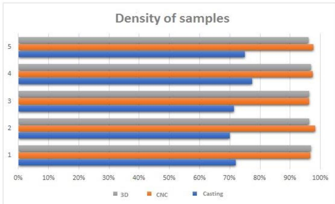
**Figure 5:** Graphic representation of density of dental restorations made by different technologies
