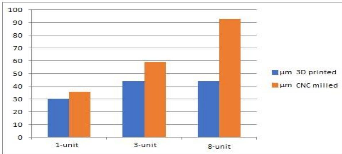
**Figure 3:** Average deviation considering the size and method of production
