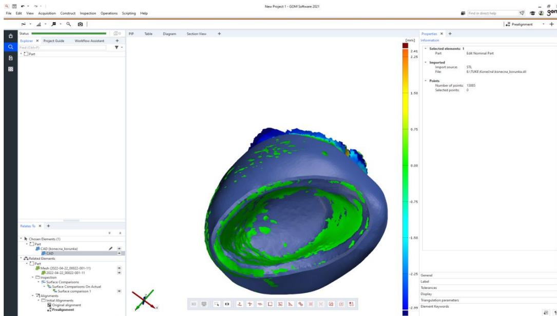
**Figure 2:** Visualization of deviation between stl. and CNC milled single crown sample made in GOMInspect software
