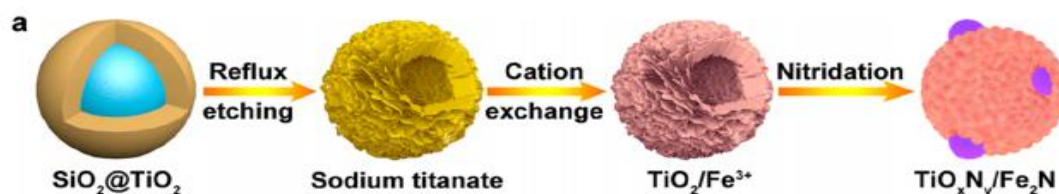
Figure 3: Schematic for the synthetic process of mesoporous \text{Fe}_2\text{N} -embedded \text{TiO}_x\text{N}_y nanoshells.
